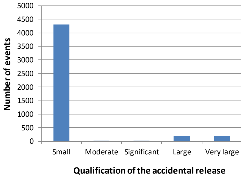
Figure 21: Intensity of offshore releases caused by accidents (source data: WOAD database, according to [12])
