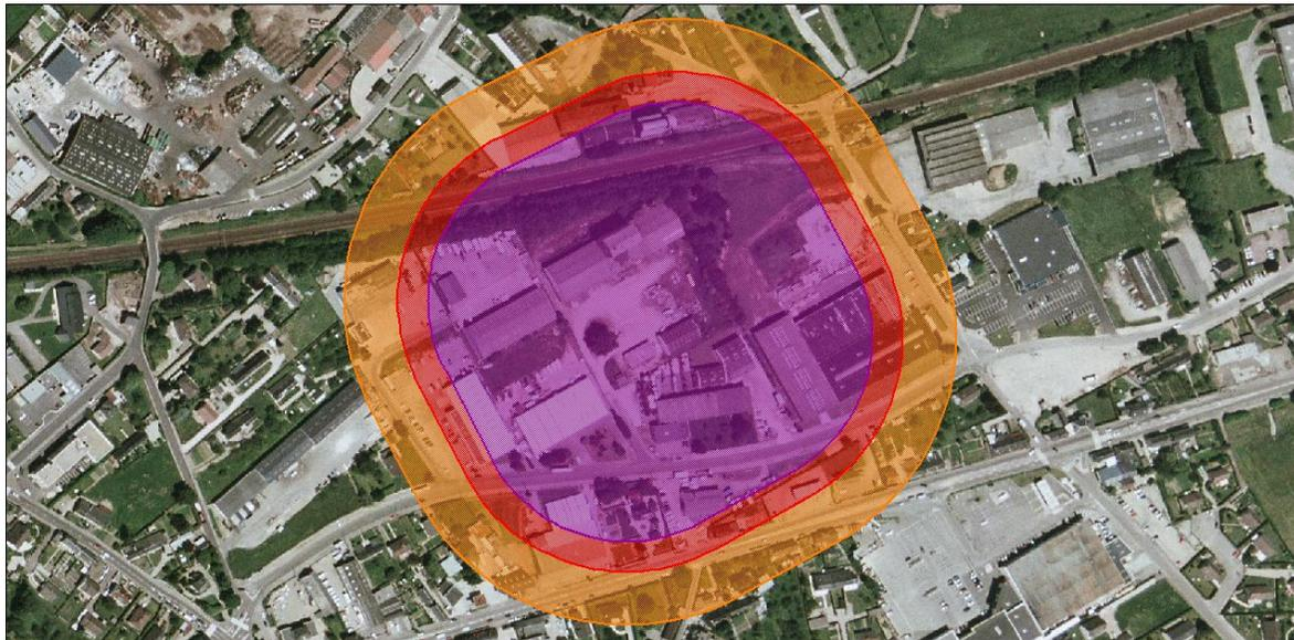
The SELS area is the purple disc, the SEL area is the red disc (union of the red crown and the purple disc), and the SEI area is the orange disc (union of the orange crown, the red crown and purple disk).
