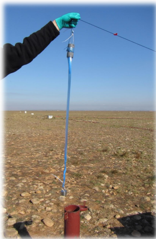
Figure 16 : Hydrasleeve™ type "SKINNY SuperSleeve 2" (source : Ineris)
