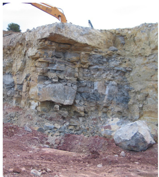
Photograph 4: Blocks broken off of rock face, Villeveyrac mining basin
