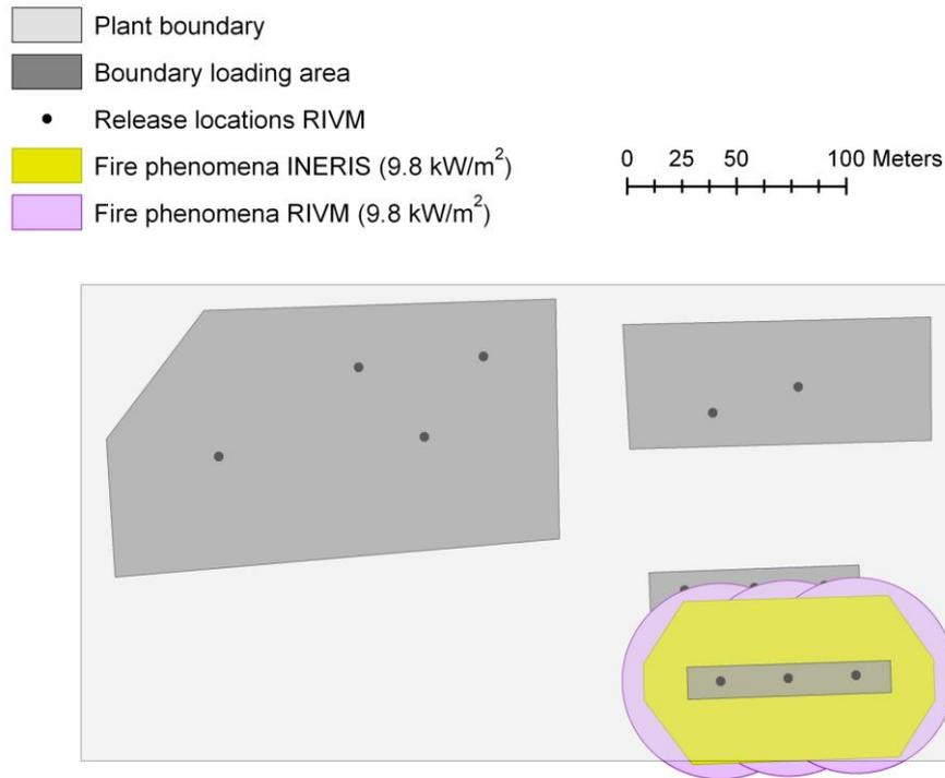
Figure 14 Fire phenomena for the loading area (weather type D5)
