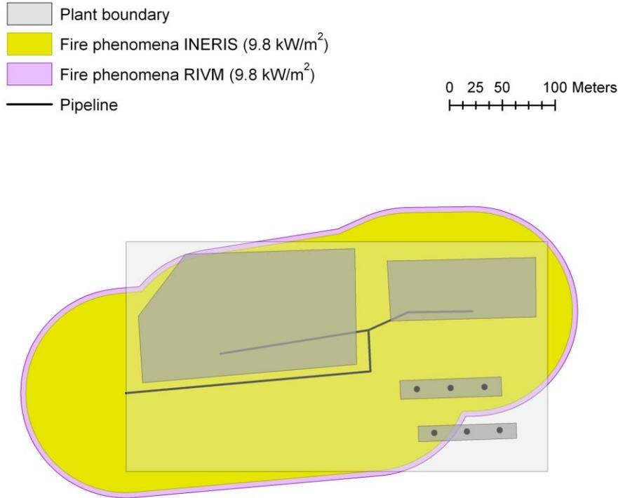
Figure 16 Fire phenomena for the pipeline (weather type D5)
