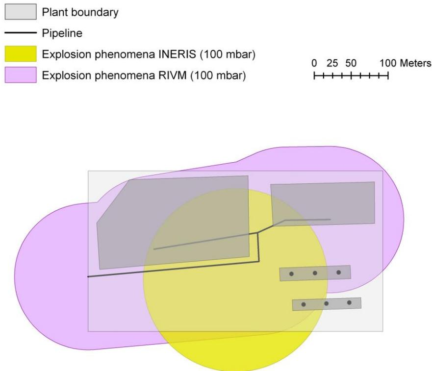
Figure 17 Explosion phenomena for the pipeline (weather type D5)
