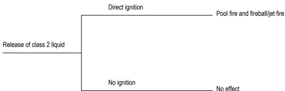
Figure 8 Event tree for dangerous phenomena following a release of class 2 flammable liquids
