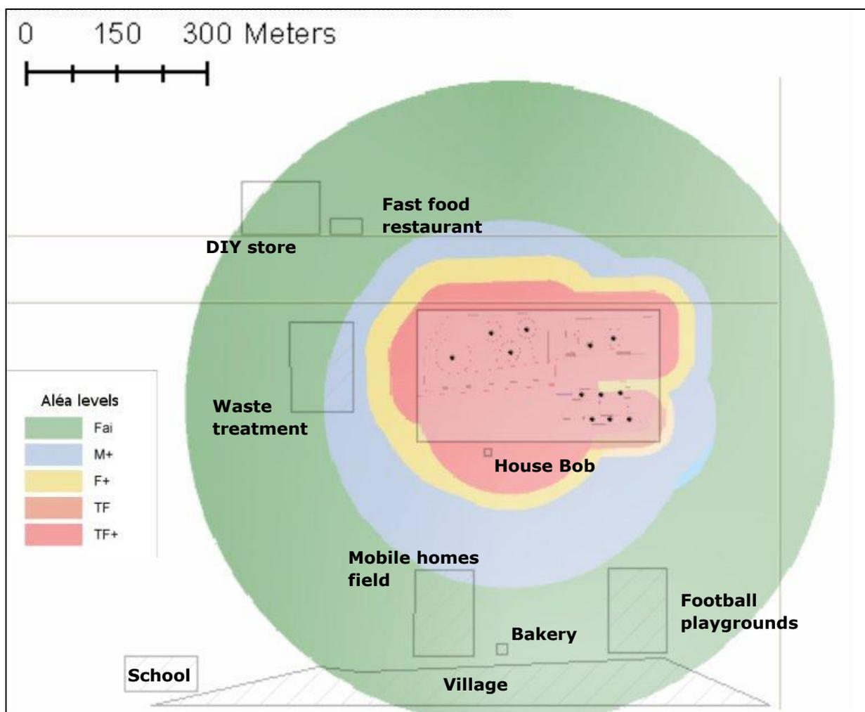
Figure 18 Synthesis of aléas without low kinetic dangerous phenomena for Fictive en Tulipes
