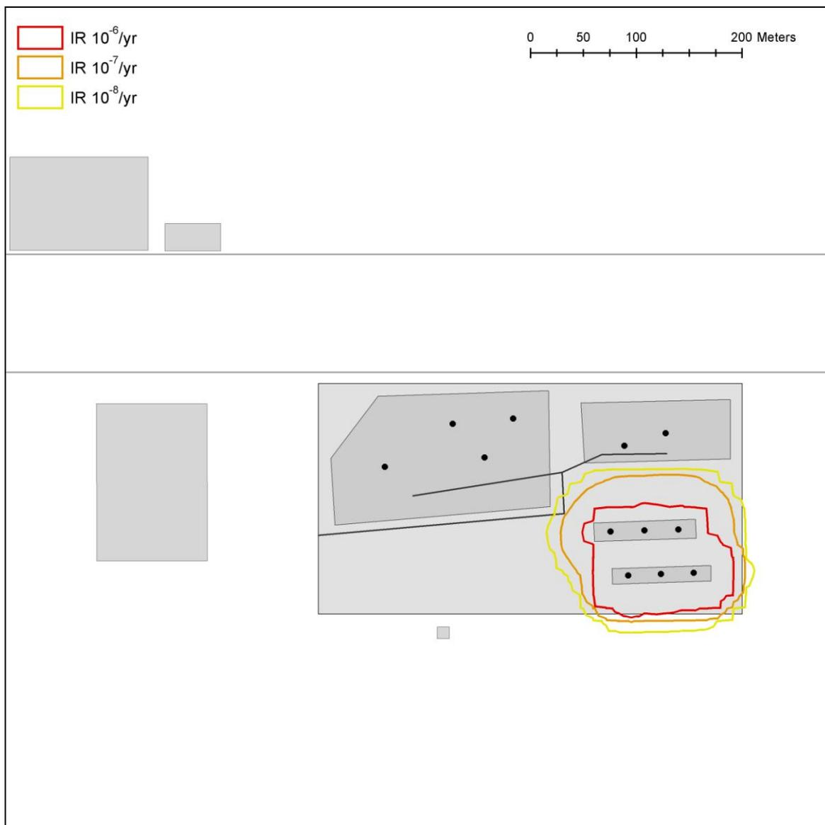
Figure 29 Individual risk contours for the pump and loading area (RIVM method)
