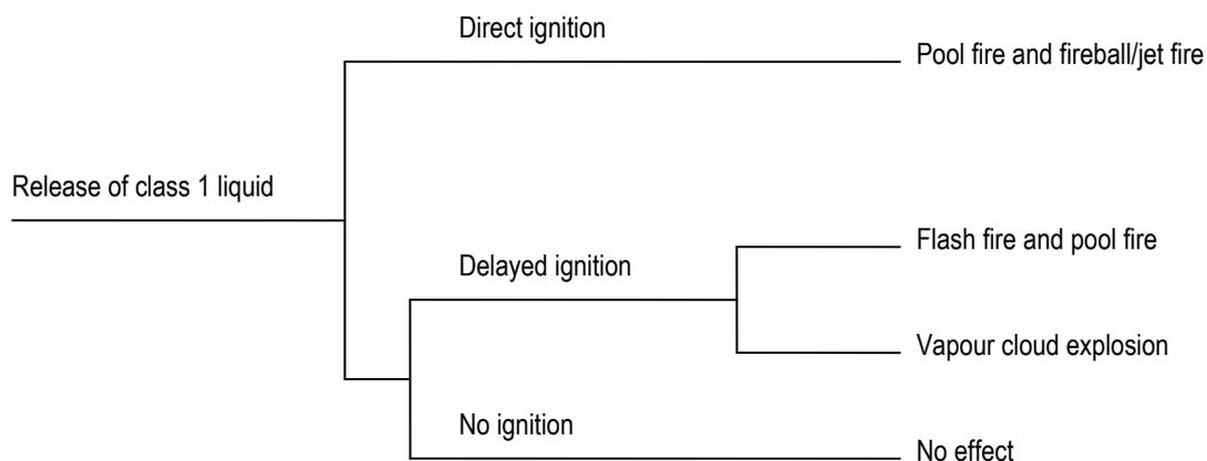
Figure 7 Event tree for dangerous phenomena following a release of class 1 flammable liquids
