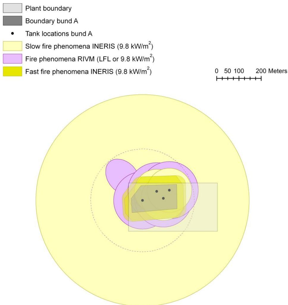
Figure 12 Fire phenomena for storage tanks in bund A (weather type D5)
