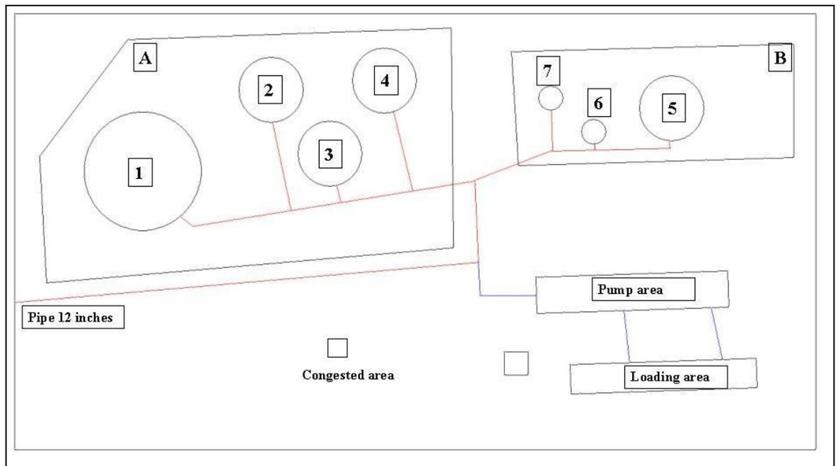
Figure 9 Layout of the flammable liquid depot
