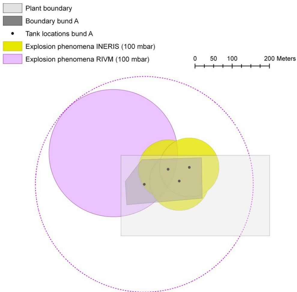
Figure 13 Explosion phenomena for storage tanks in bund A (weather type D5)
