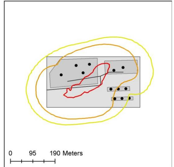
Figure 26 Individual risk contours for the entire facility, the storage area, the pump and loading area and for the pipelines (RIVM method)
