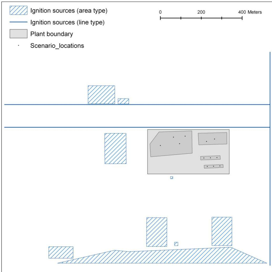
Figure 11 Ignition sources in the surrounding of the depot, as used by RIVM (ignition sources outside the facility are only relevant for societal risk, see section 2.4.2)
