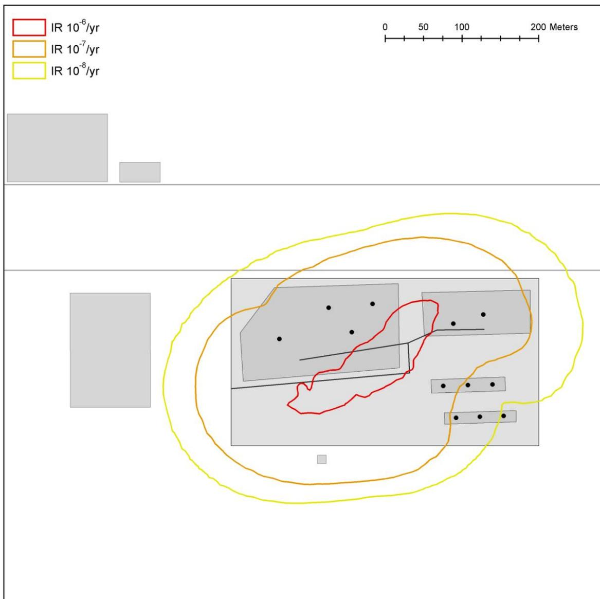
Figure 30 Individual risk contours for the pipelines (RIVM method)
