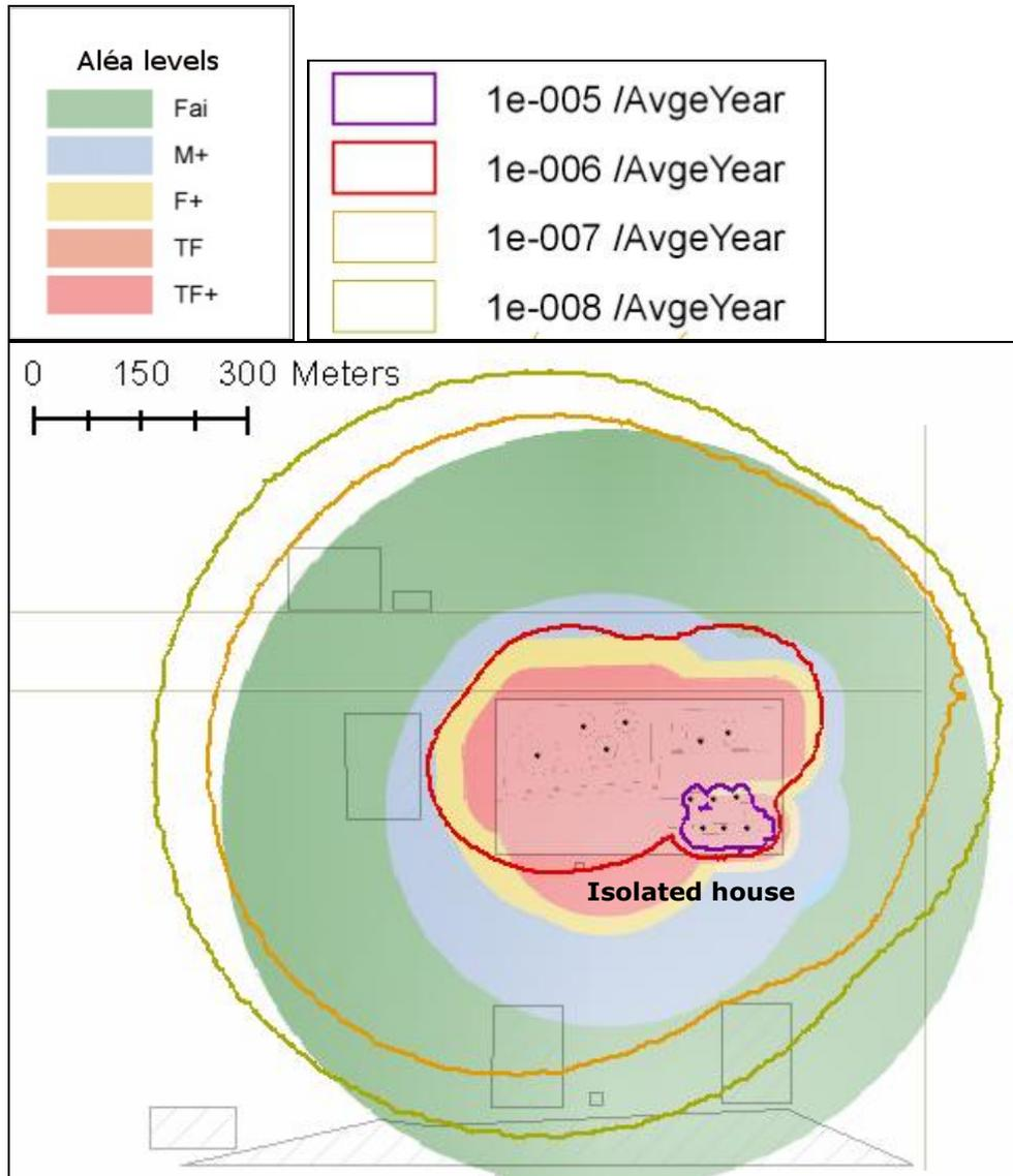
Figure 22 Dutch individual risk contours and French aléa levels for Fictive en Tulipes
