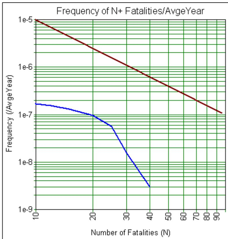
Figure 20 FN-curve for Fictive en Tulipes (Dutch methodology)
