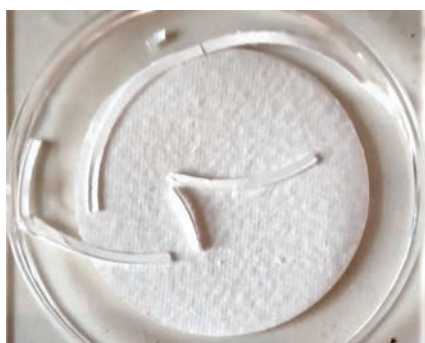
Filter deteriorated by tearing
