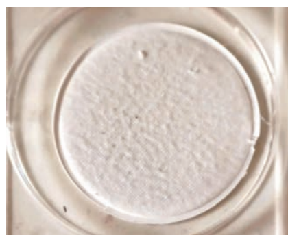
Filter deteriorated by flaking
