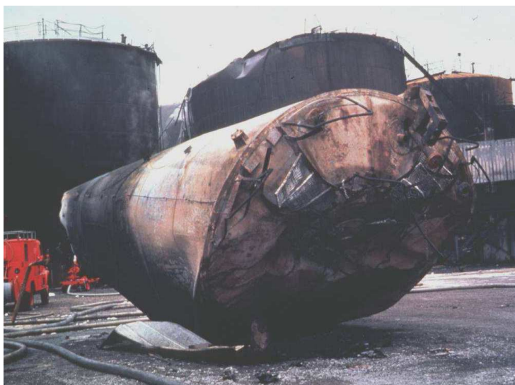
Figure 2 : Tank blown over by the explosion (ARIA sheet of the BARPI, consultable at http://www.aria.developpement-durable.gouv.fr , accident n°4998)
