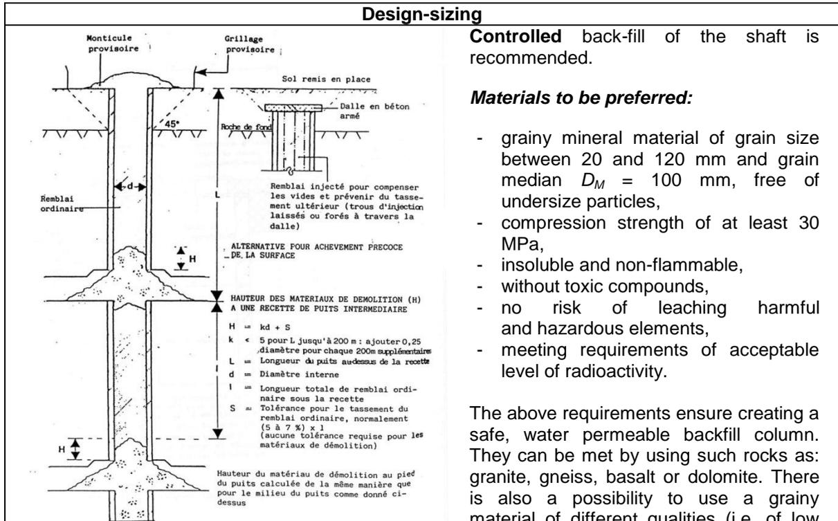
Principle of controlled back-filling of a mine shaft (National Coal Board, 1982).
