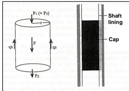
*Principle of self-supporting cap with friction (shears strength) on the shaft lining*
