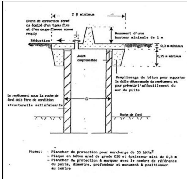
Example of outline diagram of a surface slab of the light or heavy duty type and of underground slabs installed at the top of a rocky outcrop (according to the National Coal Board)
