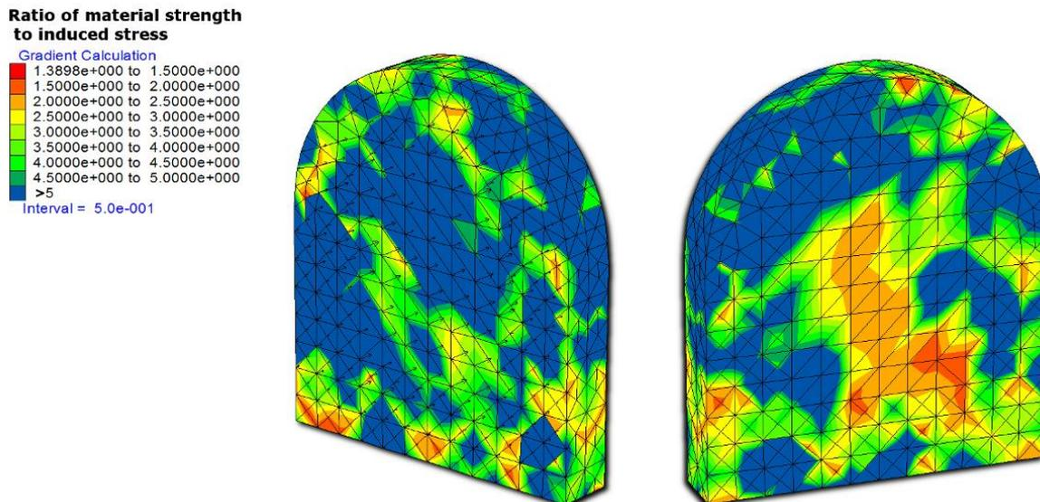
Figure 22 : Example of strength analysis using FLAC3D based on results from PFC3D
