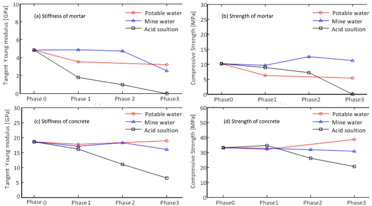
Figure 9 : UCS results for stiffness and strength change of concrete and mortar due to weathering
