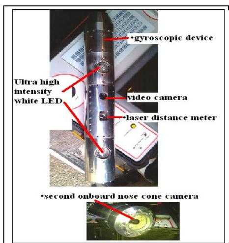
**Camera for flooded voids (probe 4)**
