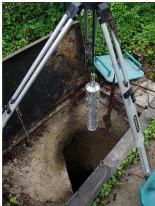
Inspection of cavities and shaft with the winder located directly at the top of the shaft or at the top of a borehole
