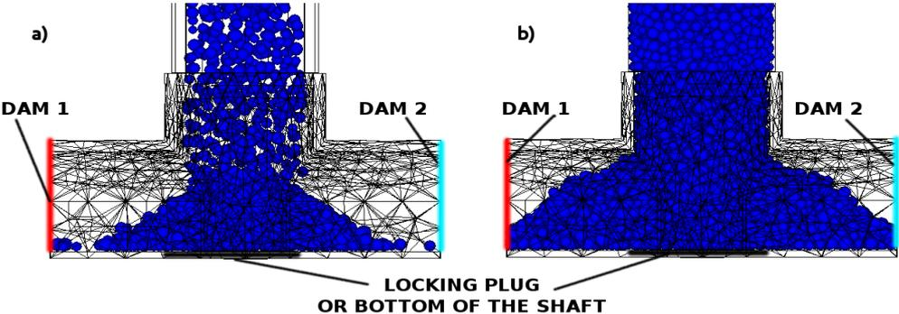
Figure 19 : Sequential stages of simulation of shaft filling – mouth view in shaft insets area.
