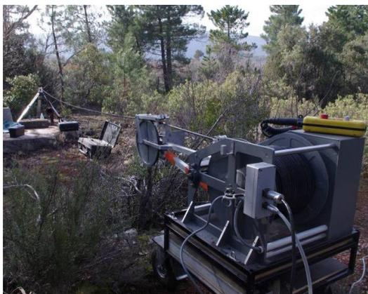
Inspection of cavities and shafts using a tripod or a deviation pulley
