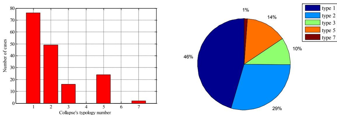
Figure 1 : The distribution of shaft failure scenarios.
