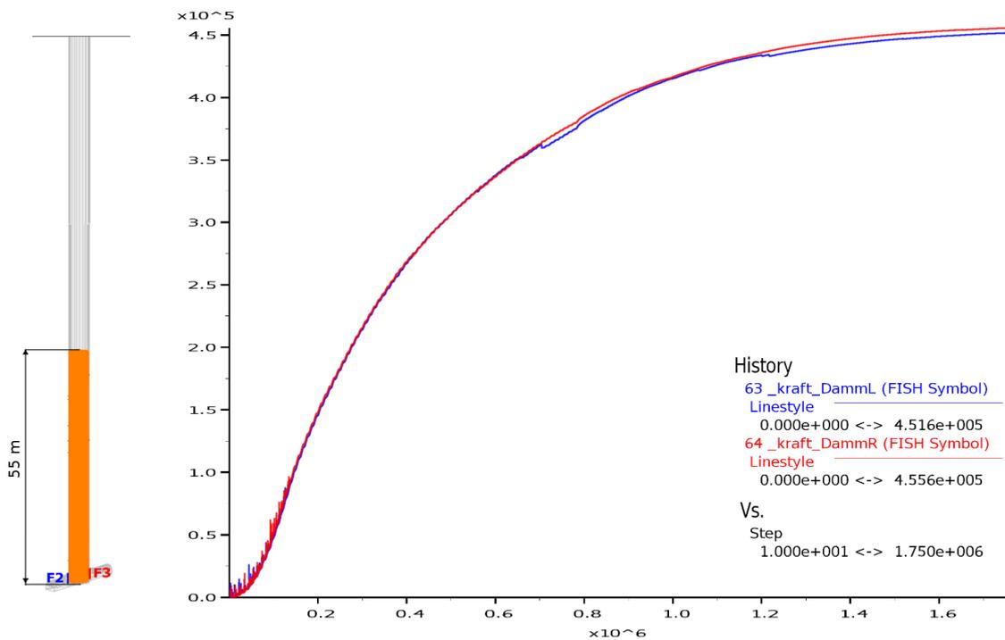
Figure 20 : Example of changes in the forces acting on the dams depending on the height of filling column
