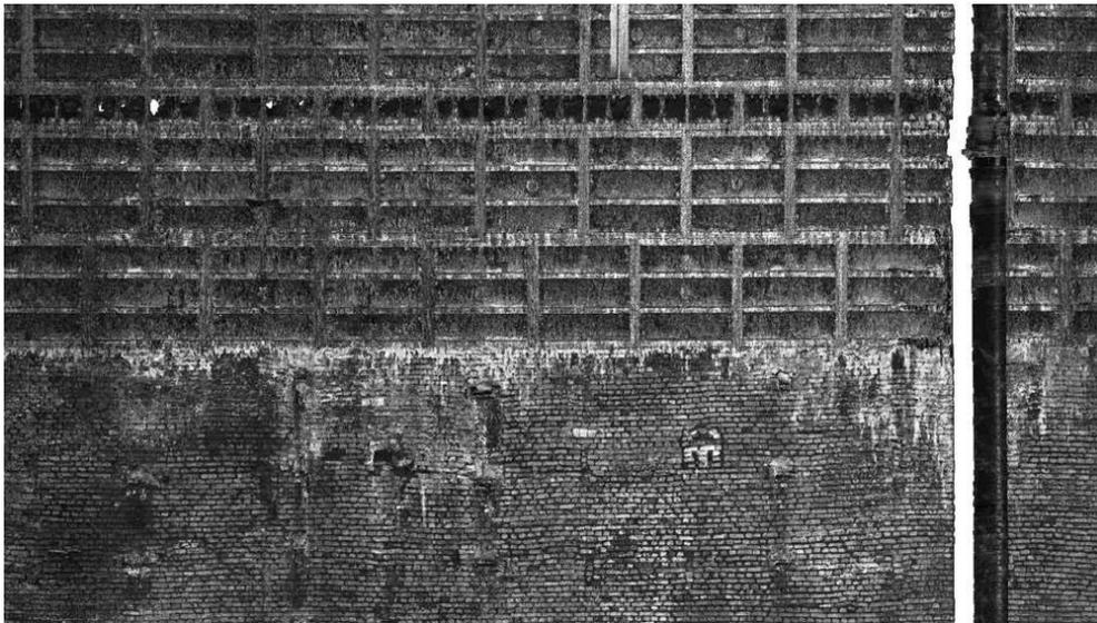
Figure 5: Unwrapped image of scan data (transmission from tubbing to brick lining)
