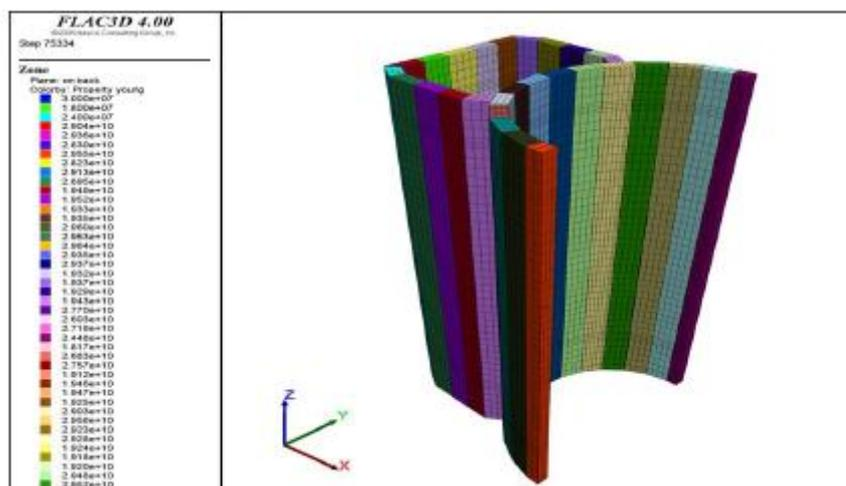
Figure 16 : Calculation model of the shaft in Flac 3D.
