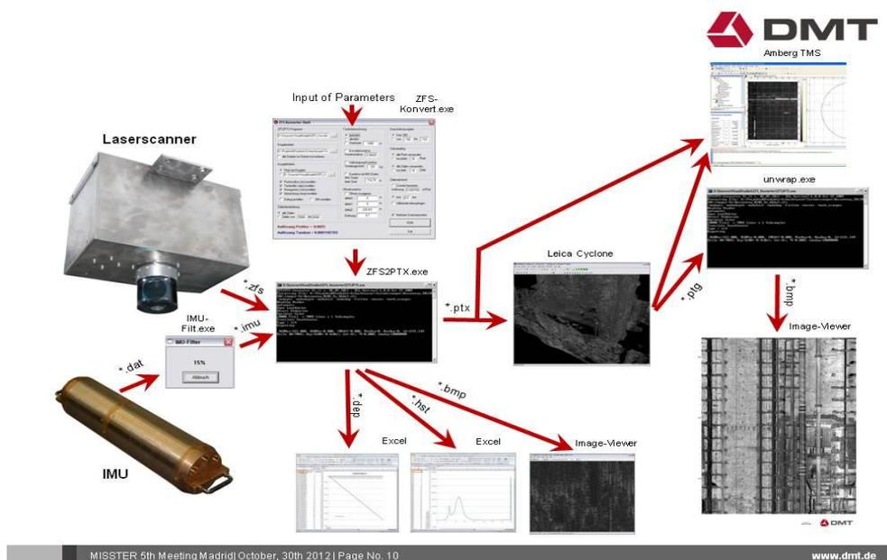
Figure 3: Workflow of data processing
