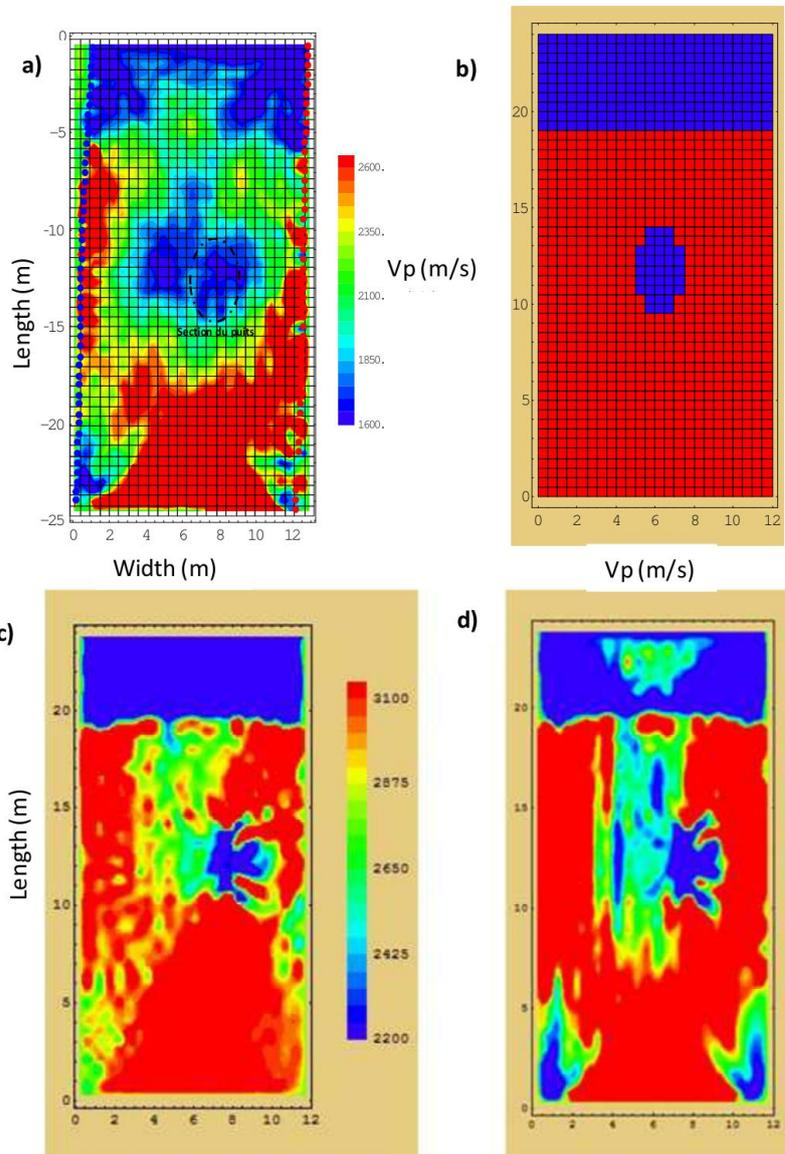
Figure 2 : Example results of mine shaft exploration using seismic tomography
