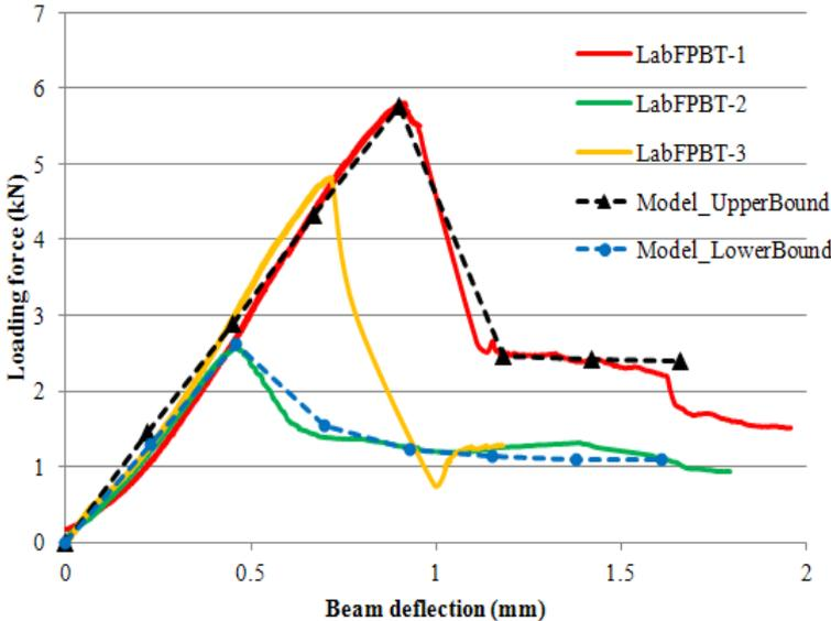
Figure 10 : Force-deflection curves for FPB on brickwork beam from numerical models & laboratory tests
