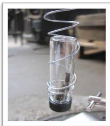
Figure 33 – BeSure<sup>®</sup> Sampler de BEACON Environmental Services Inc (source : INERIS)
