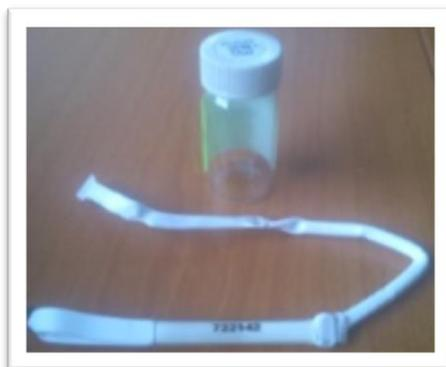
Figure 32 – Module SPG 0008® Amplified Geochemical Imaging LLC (source : INERIS)
