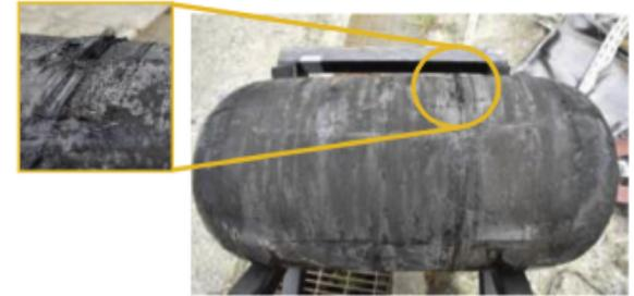
35MPa Type3,  $P_{ov}$  35MPa, Engulfing fire, Water cooling Test#10
