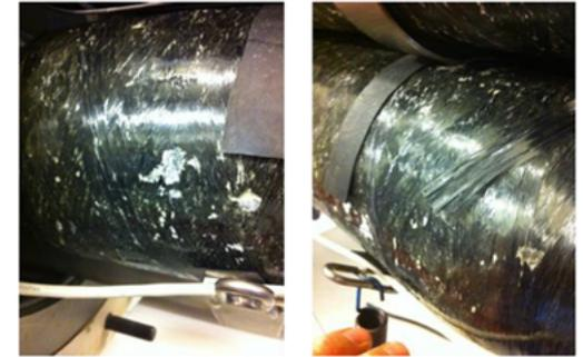
Figure 6: Two pictures of the cycled type 3 model tank's composite outer surface
