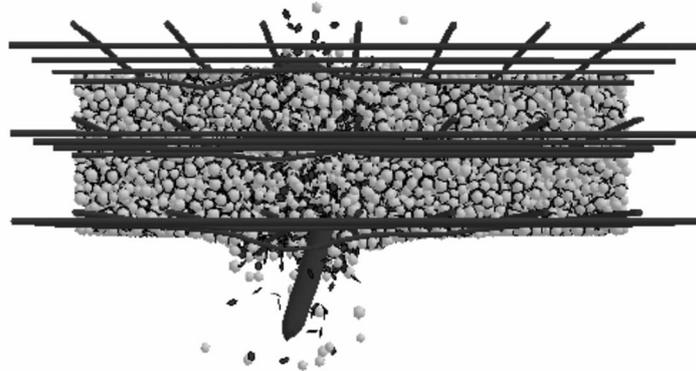
Figure 46: Simulation of the impact of a projectile on a reinforced concrete slab [Frangin 2008]
