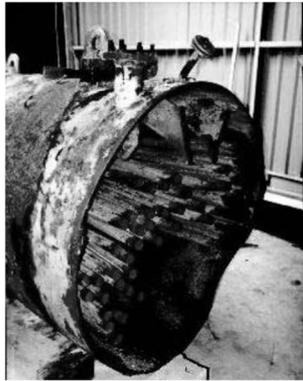
Figure 2: Boiler element propelled by rocket effect
