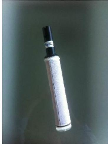
**Figure 8 : Fluxsampler Sorbisense**
