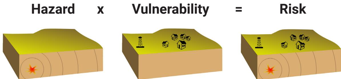
*Figure 7: Illustration of the definition of seismic risk, by the product of hazard and vulnerability*
