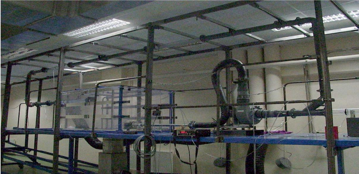
*Photo 4—2: Overview of the test dedicated to 1D/3D coupling ventilation.*
