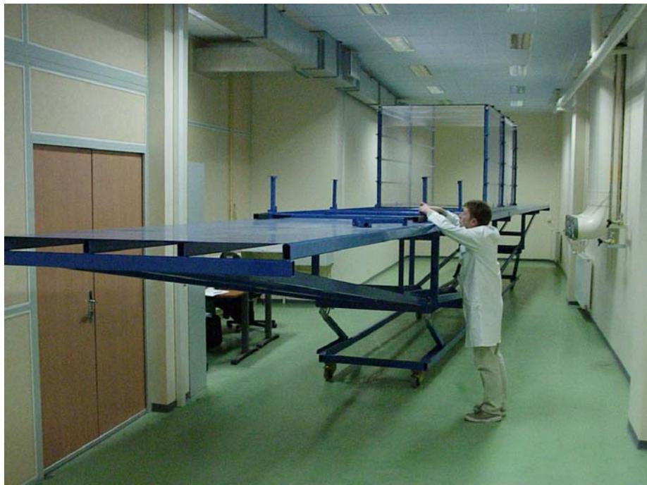
*Photo 4—1: Model facility overview showing the model base and the three-dimensional dispersion volume made up of see-through panels.*
