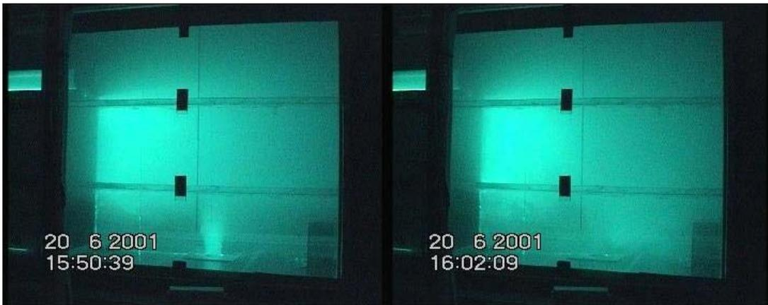
*Photo 4—5: Stratification during the stationary test phase (left) and during cell ventilation after shutting down the source (right) implying de-stratification.*
