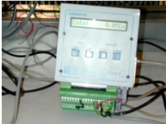
Photo n°7 : interface CENTRALP (bornier 40 points)
