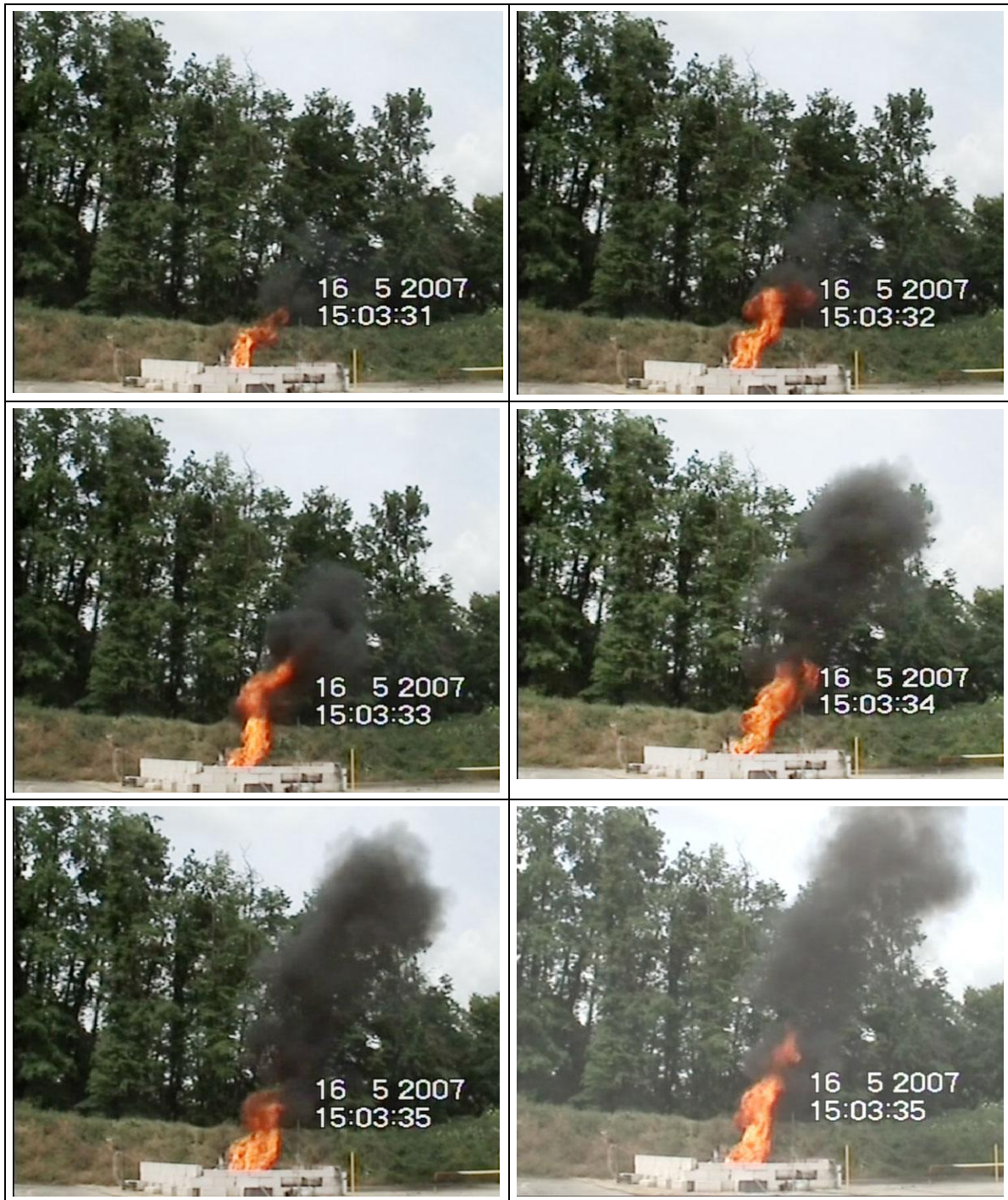
Fig. 5: Image sequence relating to the test with light crude.
