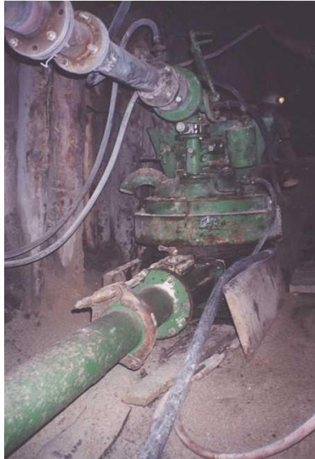
Figure 6.1. Underground stower Fig 6.2. Reinforced backfill (By courtesy of Bojan Režun)
