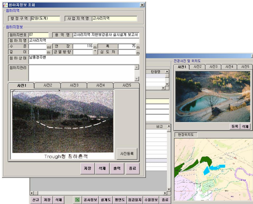
Figure 6.27. Surface subsidence control module. General information (left) and restoration work history (right) (Lee et al., 2005).
