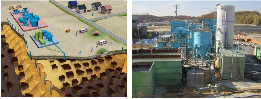
Figure 2.12. Illustration and application of backfilling technique (source Tobishima Co.).
