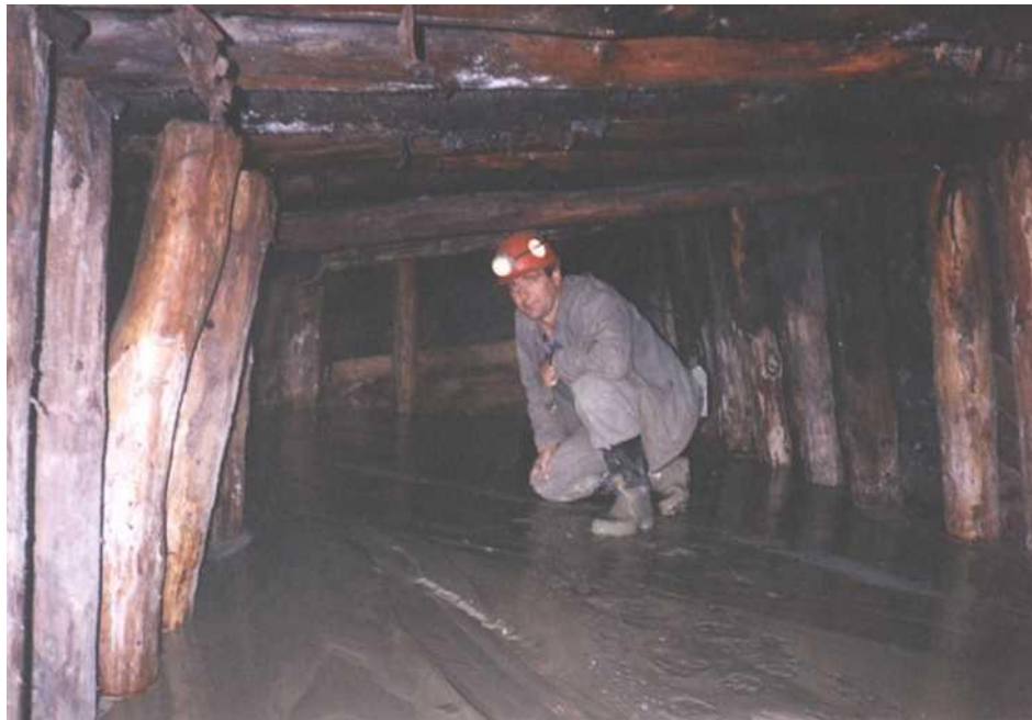
Fig. 6.5. Injected paste in abandoned underground area (By courtesy of Bojan Rezùn).
