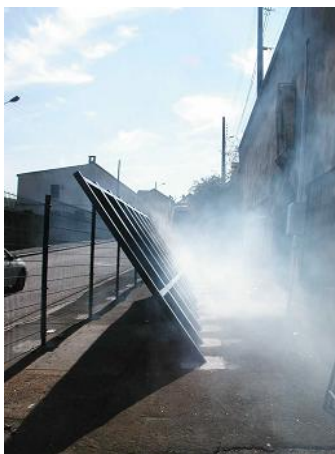
Figure 2.10. Gas emission on surface through an adit. Fumes are used to show gas flow (source INERIS).
