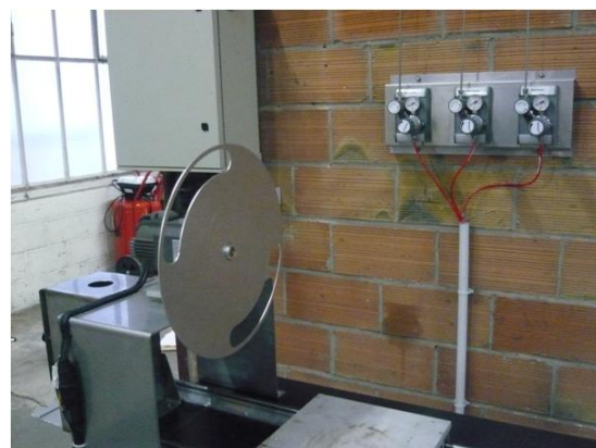
Picture 3: Combustion chamber & rotating chopper disc
