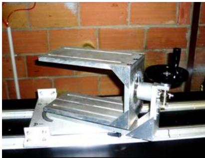
Figure 6: Rotating device for angle \alpha determination (from -65^\circ to +65^\circ )
