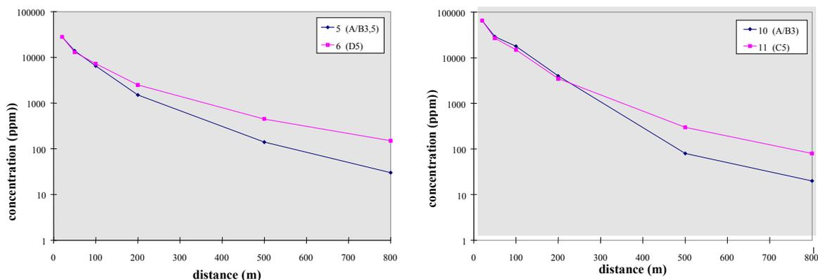
figure 24: Progression of concentrations on release axis as a function of distance for different weather conditions.
