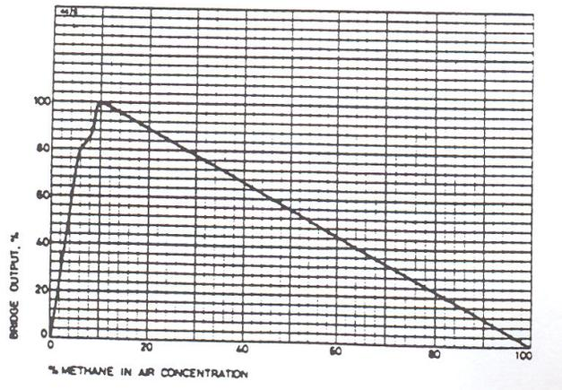
Figure 2.3: Pellistor type sensor output signal for exposure to methane
