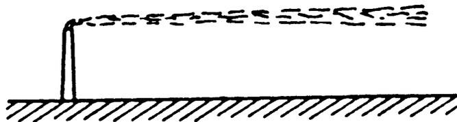
figure 14: Dispersion in a stable atmosphere (taken from Pasquill, 1974)
