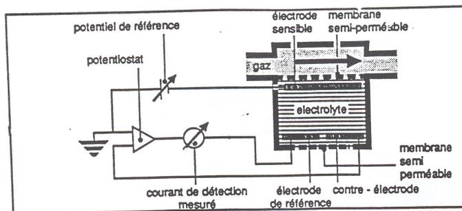
Figure 2.1: Functional description of an electrochemical cell (diagram p 44 fig. 5 in CECA report [1])
