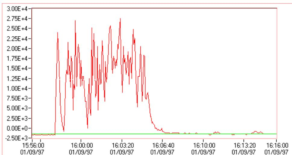
*figure 17: Progression over time of ammonia concentration (in ppm) 100 m from release point observed during test 2.*
