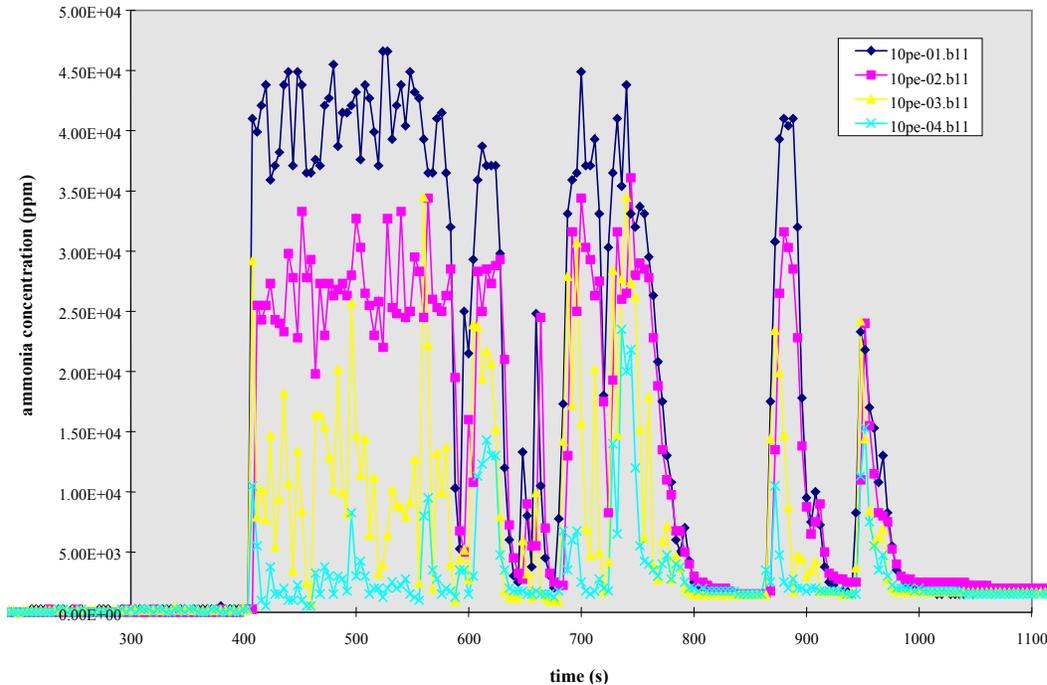
*Legend '10pe-01.b11': The first number '10' corresponds to the trial number, the two letters 'pe' (or 'tc' or 'ec') corresponds respectively to the sensor type (pellistor, thermocouple or electrochemical cell), the number '01' corresponds to the height level, and the extension corresponds to the mast number.*
