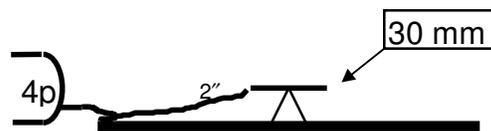
Horizontal release at a height of 1 metre via a 30 mm orifice.
