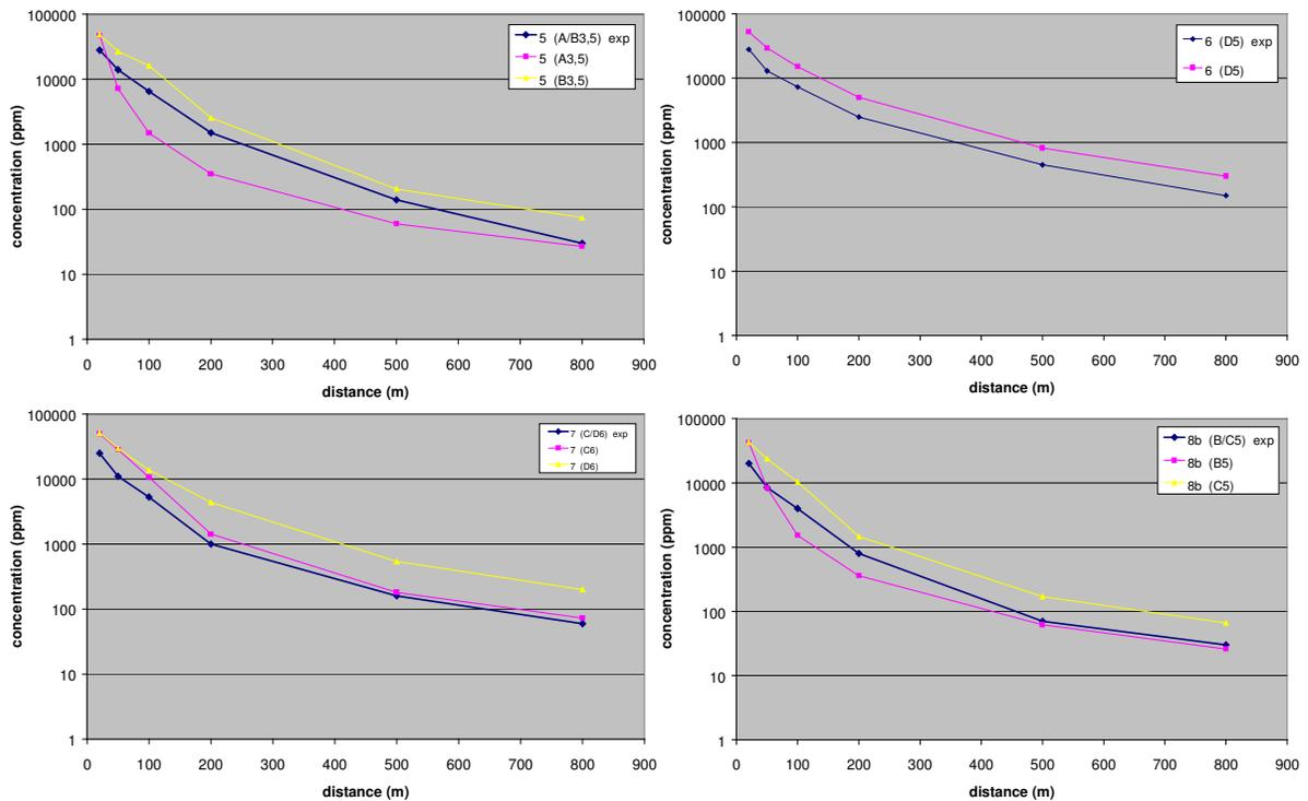
figure 31: Comparisons between calculation results and experimental results for tests 5, 6, 7 and 8b
