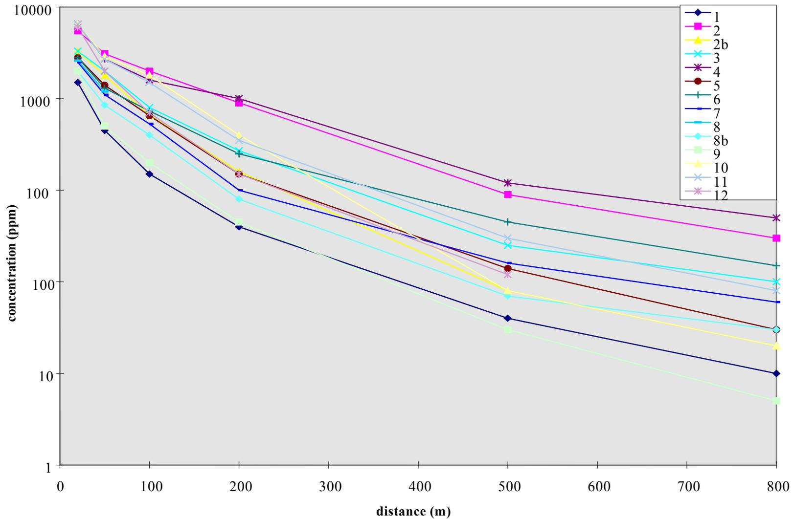
figure 19: Progression of ammonia concentrations on plume axis as a function of distance to release point
