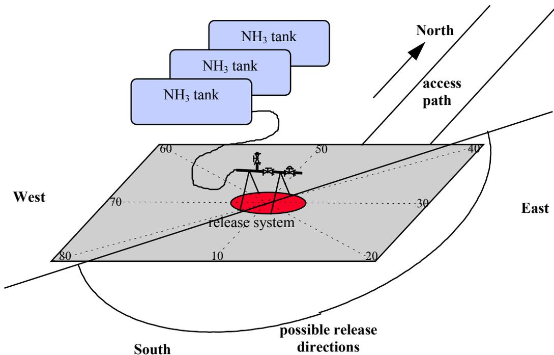
figure 10: Identification of angles on release slab
