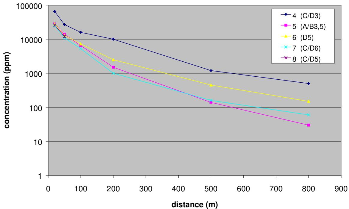
figure 27: Progression of concentrations as a function of distance for tests 4, 5, 6, 7 and 8.
