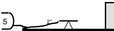
Horizontal release at a height of 1 metre impacting a wall with a surface area of 3 m x 3 m. This wall is located 3 m from the end of the release system.
