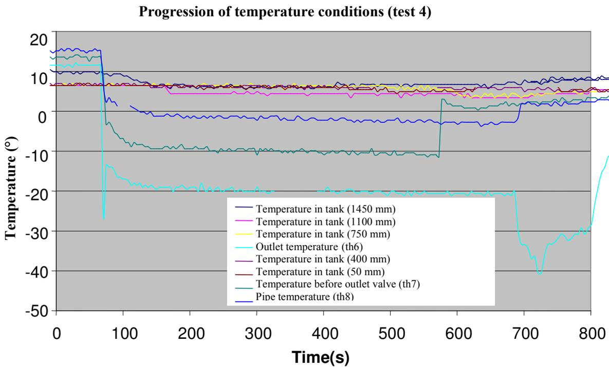
figure 12: Progression of pressure and temperature conditions in tank and in release pipe
