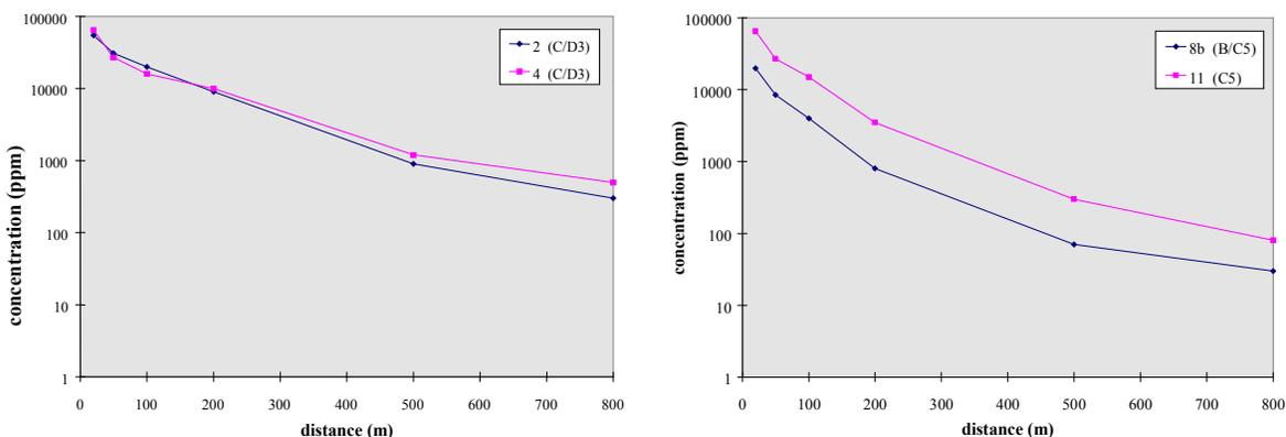
figure 25: Progression of concentrations on release axis as a function of distance for similar weather conditions.
