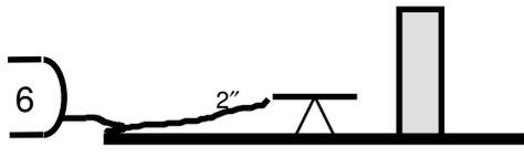
Horizontal release at a height of 1 metre impacting a wall with a surface area of 3 m x 3 m. This wall is located 1 m from the end of the release system.
