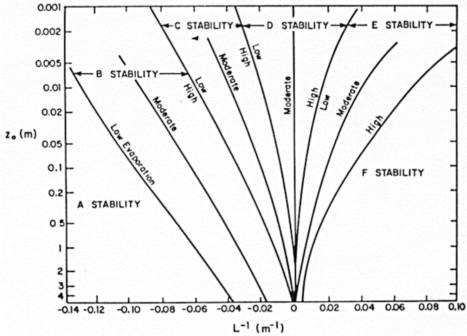
figure 15: Relationship between the Monin-Obukhov  $L$  and the roughness  $z_0$  for different Pasquill stability classes (Golder, 1972).
