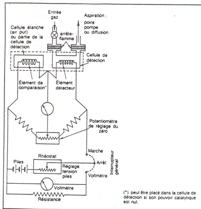
Figure 2.2: Principle diagram of catalytic oxidation measurement device (INRS diagram)
