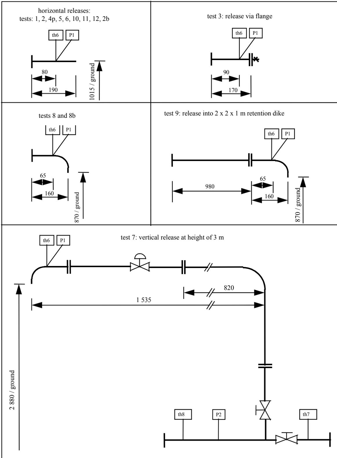
figure 5: different outlet types for each configuration
