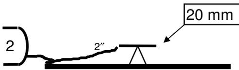
Horizontal release at a height of 1 metre in liquid phase via a 20 mm orifice.
