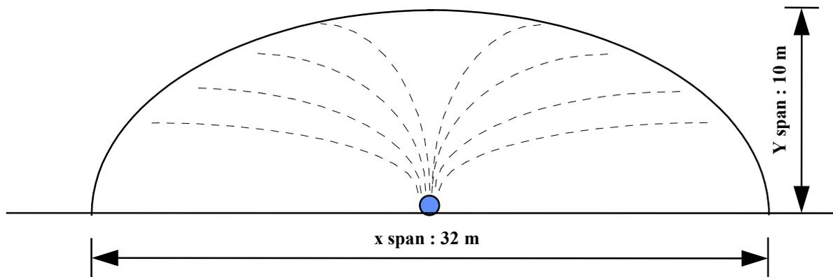
*figure 6: spans of peacock tails used for tests 10 and 11.*
