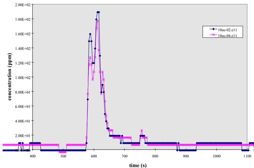
figure 22: Progression of ammonia concentration values for sensors located on the same mast 500 metres from the release point
