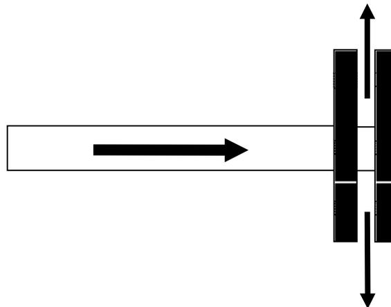
figure 2: Diagram of device used to simulate a leakage on a flange.
