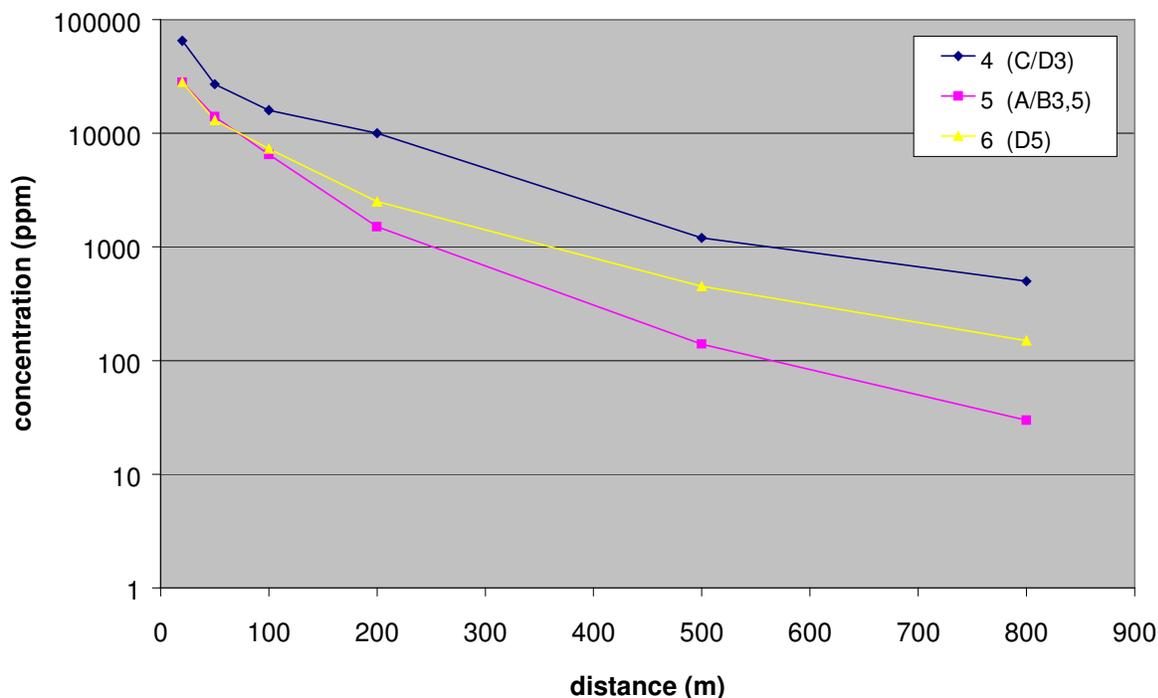
figure 26: Progression of concentrations as a function of distance for tests 4, 5 and 6
