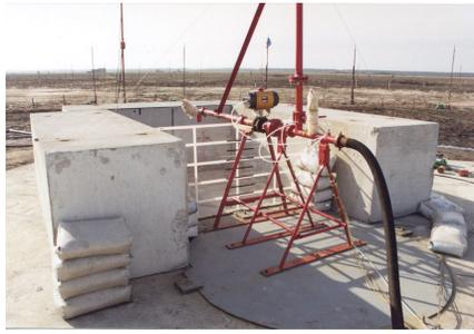
photo 4: Vertical release in a 4m<sup>3</sup> retention dike
