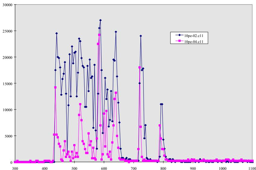
figure 21: Progression of ammonia concentration values for sensors located on the same mast 100 metres from the release point
