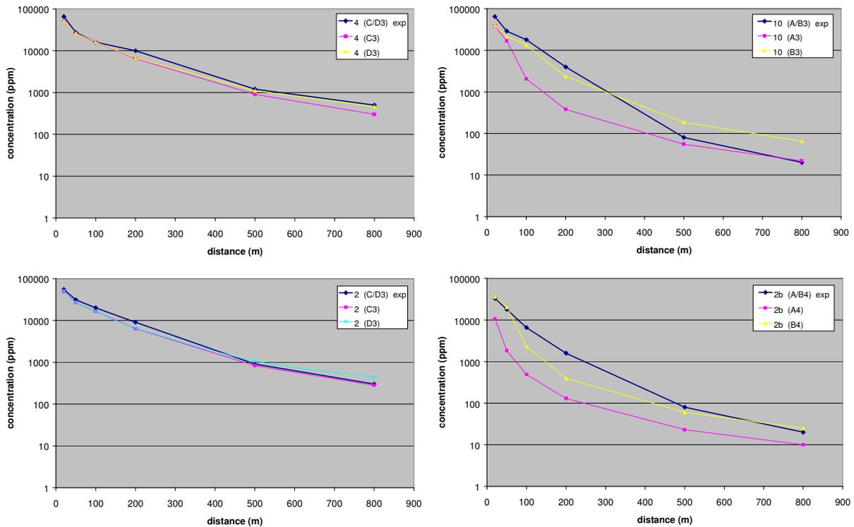
figure 30: Comparisons between calculation results and experimental results for tests 4, 10, 2 and 2b
