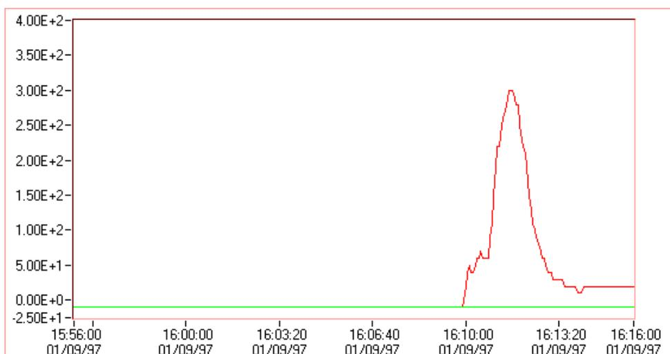
figure 18: Progression over time of ammonia concentration (in ppm) 800 m from release point observed during test 2.
