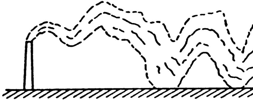
figure 13: Dispersion in an unstable atmosphere (taken from Pasquill, 1974)
